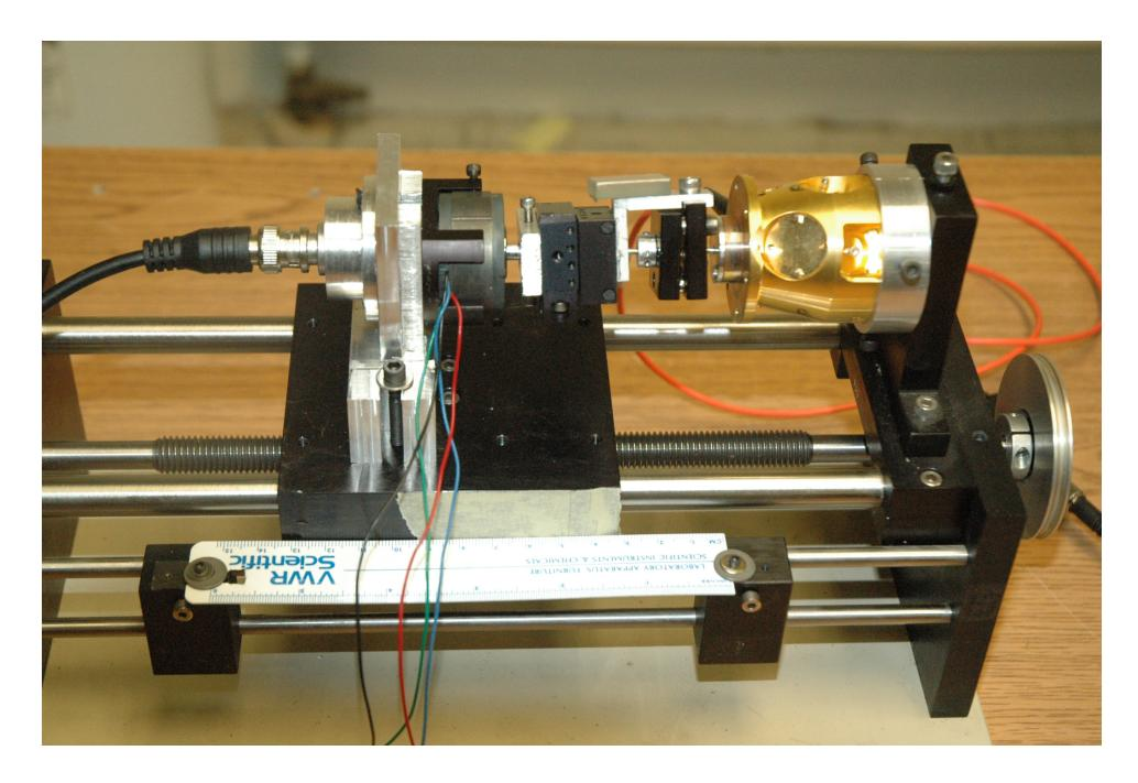
Laser light of wavelength 635 nm is directed into the spherical cavity from a DFB laser source. Reflected light enters a small prism at the end of a fiber optic periscope and is measured by a photodiode at each position. The periscope is rotated in 0.9 deg increments using a stepping motor and Labview software to obtain data for one complete revolution. The periscope is translated in the z direction in 1 mm increments to record data sets for 20 z positions.
