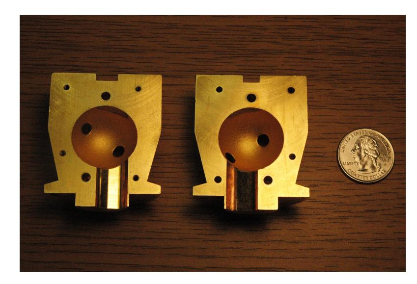
The inner walls of the layering sphere are covered with a rough gold coating to produce Lambertian scattering. There are various windows that can be covered with flanges.
