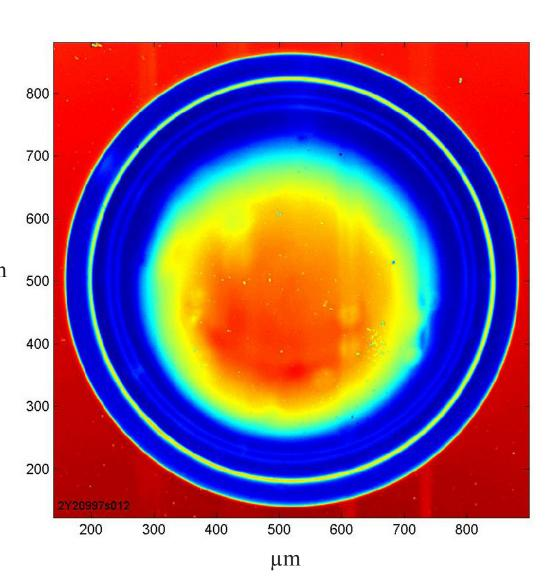
To improve the uniformity of the ice layer, the DT target is placed in the center of a spherical cavity called a layering sphere and is illuminated with infrared light, promoting ice sublimation.
