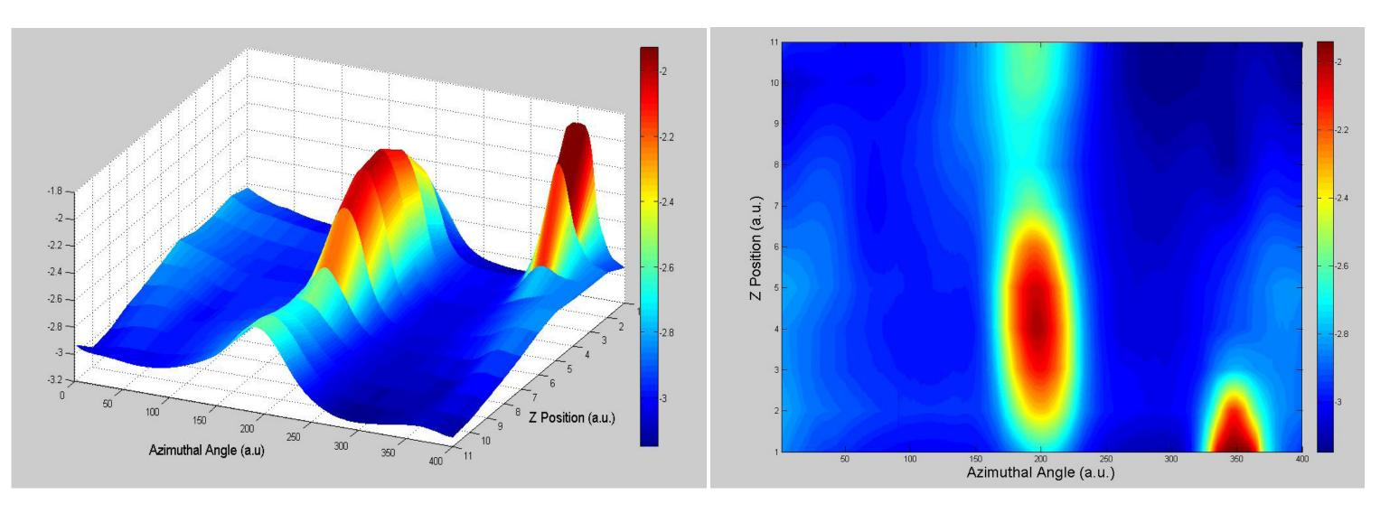
3 dimensional representation of signal intensity. The data on the left was taken with the windows removed. The images below are the same data viewed from the opposite side. The top two images display the laser entry point while the lower two show the initial bright spot.
