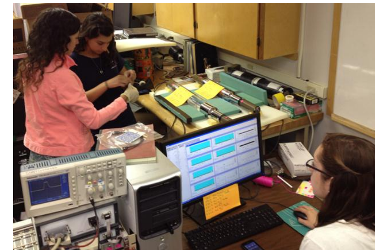
Two pairs of 3 inch by 3 inch NaI detectors were used for coincidence counting
