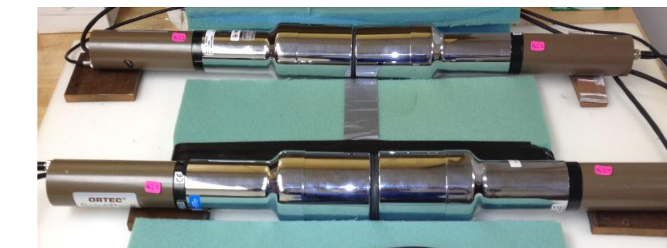
Two pairs of 3 inch by 3 inch NaI detectors were used for coincidence counting
