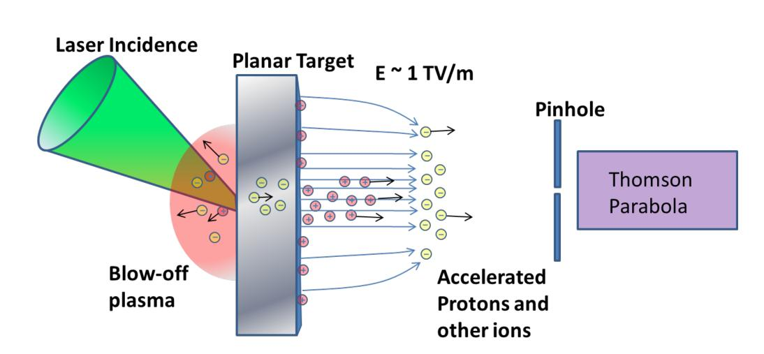
A Thompson Parabola Ion spectrometer designed and built at SUNY Geneseo was used to analyze the Electrons and Ions. A Thompson Parabola consists of a set of magnetic field plates and electrical field plates that bend the ions and electrons according to their charge to mass ratio and energy. The electric field plates were left off for this experiment.
