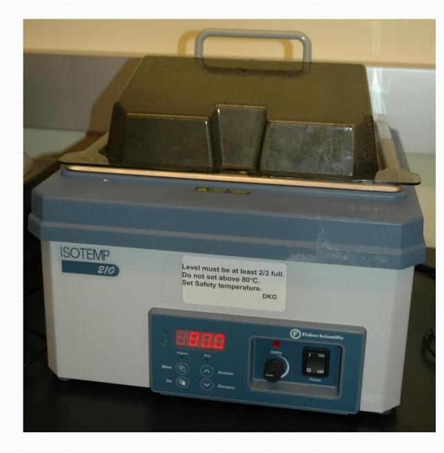
Both pieces are etched in 6N NaOH for six hours at 80°C in the same beaker. Then they are both rinsed with tap water and air dried overnight
