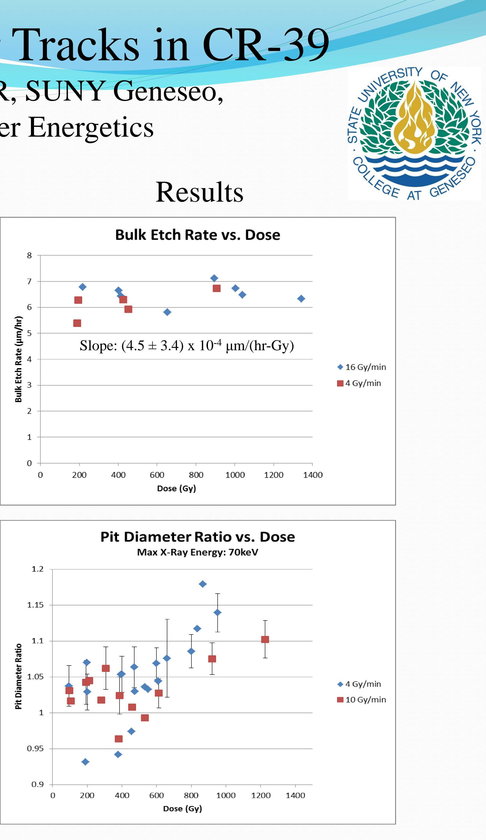
Our results showed little correlation between bulk etch rate and x-ray dose; however, pit diameters increased with increasing x-ray dose. The enhancements measured were modest; only a 10% increase in pit diameter was observed after an x-ray exposure of over 3 hours.
