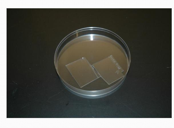
Side A is exposed to x-rays and the dose is measured while Side B is stored at STP
