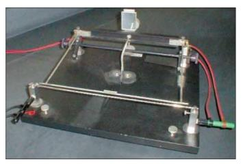
Fig. 1. The current balance. With identical current flowing in opposite directions through the top, moveable wire and the bottom, stationary wire, the top wire will rise slightly.
