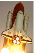
jettisoned and land in the ocean. They are retrieved by special ships and reused. The cryogenic fuel tank is connected to the Orbiter for about ten minutes. It carries the fuel (at a temperature of less than  $-200^{\circ}$ C) for the three main engines on the back of the Orbiter (but not for the booster rockets). Once emptied, it is jettisoned and burns up in the atmosphere.
