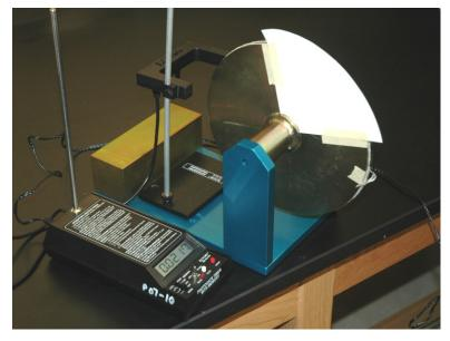
To measure m, we will first determine the density  $\rho$  of this material (steel) using a reference brick as seen here. You will need to weigh the brick, and also you'll need to determine its dimensions.
