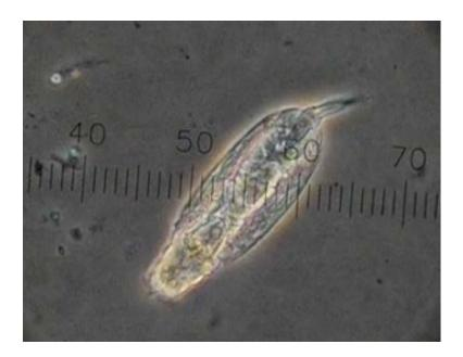
3. Next I should add a scale bar. I know that between each of the eyepiece lines is 2.5 uM (since I took this at 40X), so I can add an appropriate scale bar by putting in a line with a known distance (this line spans 4 eyepiece micrometer lines, so it's 2.5\*4=10 um).
