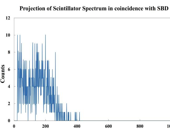
The neutron time of flight was determined by examining shifts in the TAC spectra as the scintillator was moved different known distances from the target chamber. The neutron velocity was found to be  $(2.099 \pm 0.014) \times 10^7$  m/s. After calculating the neutron velocity, the neutron energy was determined to be  $2.30 \pm 0.31$  MeV, which is consistent with the predicted neutron energy, 2.595 MeV. This confirms the APT is selecting only d-d fusion neutrons.
