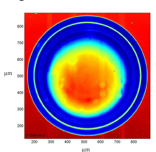
To improve the uniformity of the ice layer, the DT target is placed in the center of a spherical cavity called a layering sphere and is illuminated with infrared light, promoting ice sublimation.
