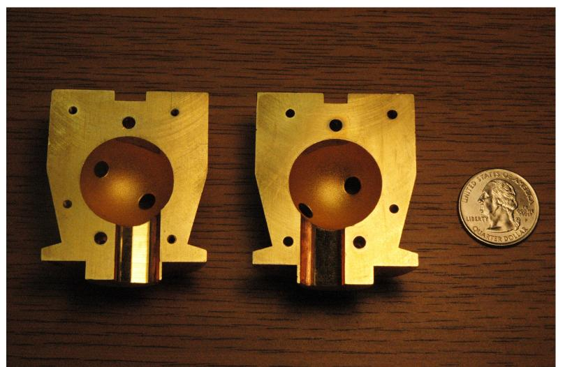
The inner walls of the layering sphere are covered with a rough gold coating to produce Lambertian scattering. There are various windows that can be covered with flanges.
