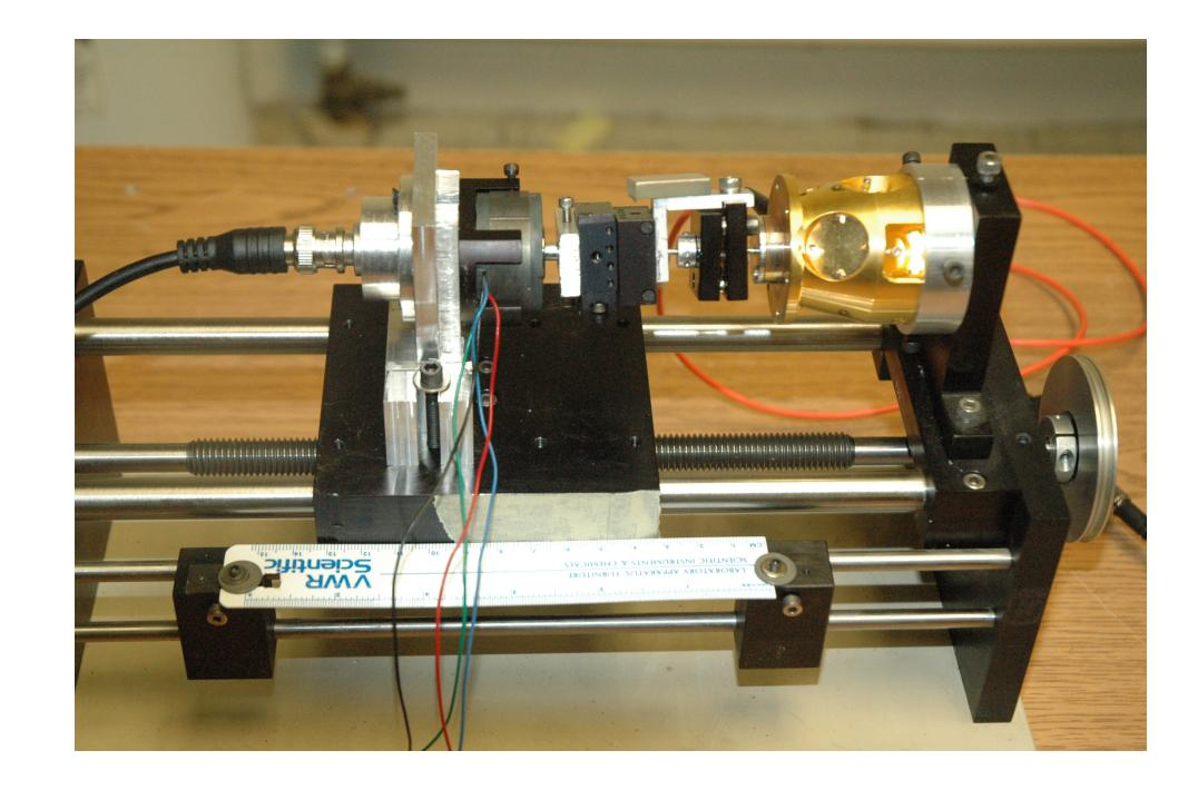
Laser light of wavelength 635 nm is directed into the spherical cavity from a DFB laser source. Reflected light enters a small prism at the end of a fiber optic periscope and is measured by a photodiode at each position. The periscope is rotated in 0.9 deg increments using a stepping motor and Labview software to obtain data for one complete revolution. The periscope is translated in the z direction in 1 mm increments to record data sets for 20 z positions.
