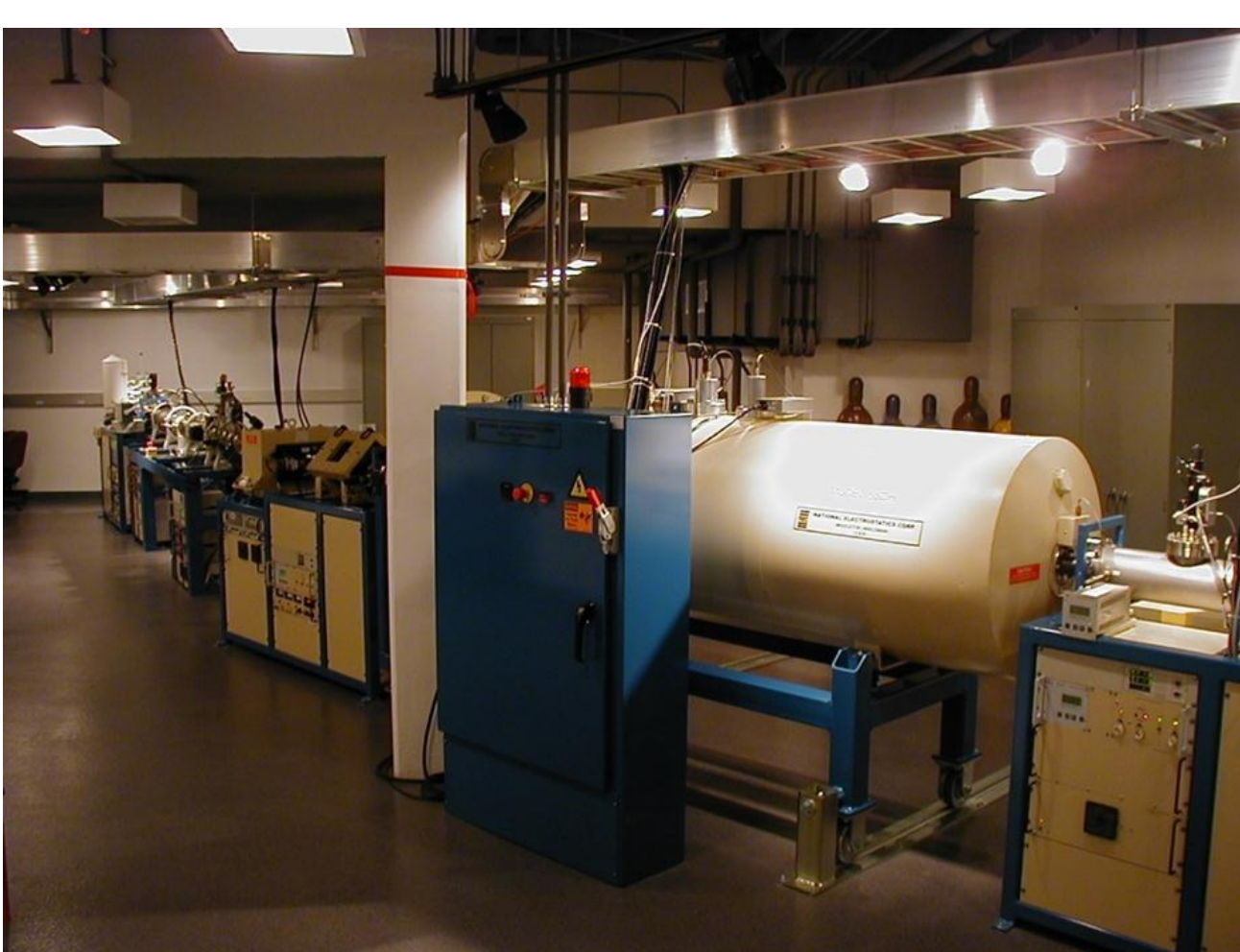
(Left) A picture of the accelerator beam line. (Right) A schematic depicting the 15R beamline and end station of Geneseo's 1.7 MV tandem Pelletron accelerator for the activation of ^{11}\text{B} .
