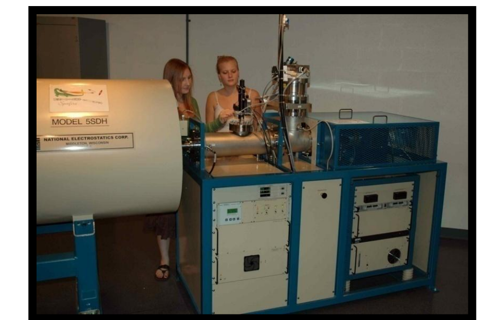
View of the source on the 1.7 MV Tandem Pelletron accelerator
