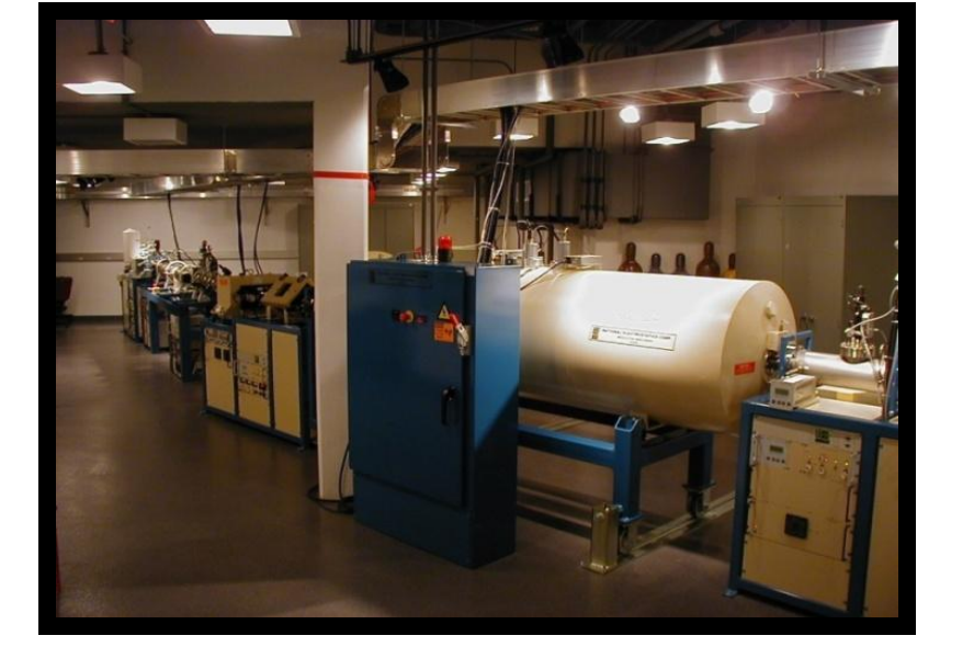
View of the source on the 1.7 MV Tandem Pelletron accelerator
