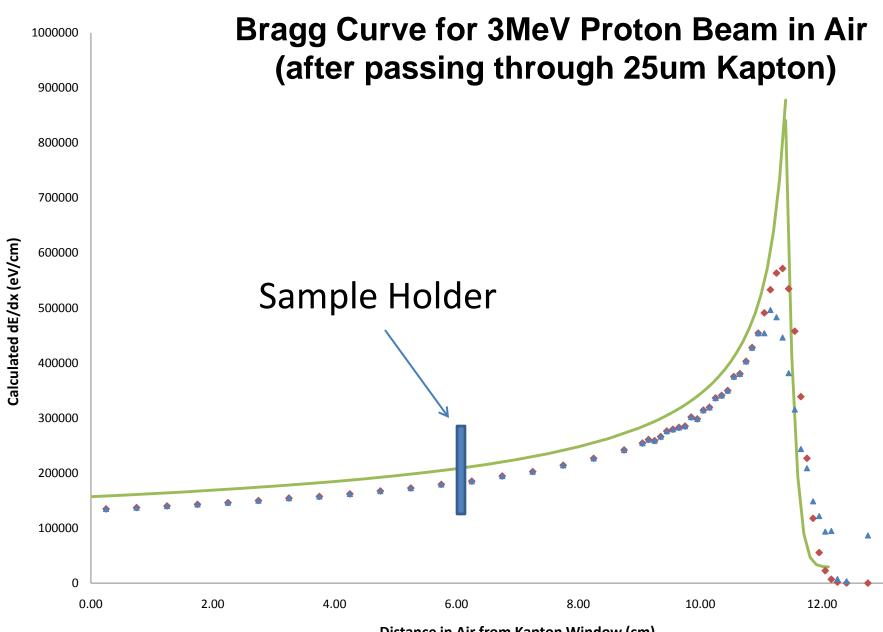
Proton energy loss and beam straggling through Kapton and air were determined theoretically using TRIM tables and SRIM calculations. These were confirmed by calibration experiments using time exposure photography and Radiochromic Film.
