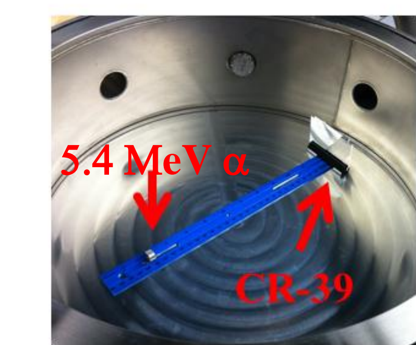
Alpha Particle Irradiation 2 hours in vacuum
