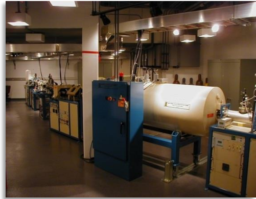
Figure 3: The new 1.7 MV Pelletron accelerator at SUNY Geneseo, installed in 2007.
