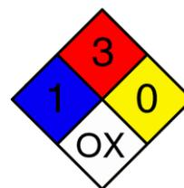
8.4.2 The hazard identification signal is a color-coded arrangement of numbers and/or letters arranged in a diamond shape. NFPA Hazard diamonds are displayed on any container which stores or transports hazardous chemicals, including trucks, storage tanks, bottles of chemicals, and in various other places. The blue, red, and yellow fields (health, flammability, and reactivity, respectively) all use a numbering scale ranging from 0 to 4.
