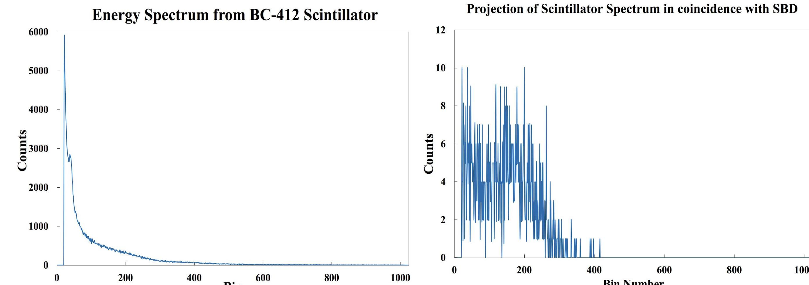
The neutron time of flight was determined by examining shifts in the TAC spectra as the scintillator was moved different known distances from the target chamber. The neutron velocity was found to be  $(2.099 \pm 0.014) \times 10^7 \text{ m/s}$ . After calculating the neutron velocity, the neutron energy was determined to be  $2.30 \pm 0.31 \text{ MeV}$ , which is consistent with the predicted neutron energy, 2.595 MeV. This confirms the APT is selecting only d-d fusion neutrons.
