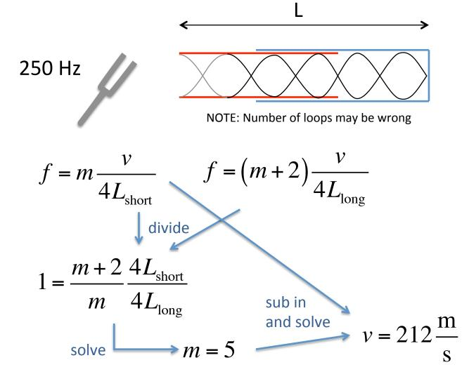
Sound from tube is especially loud for lengths L=1.06m and L=1.48m
