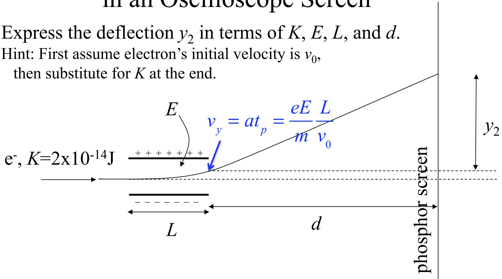
$$\text{horizontal: } t_d = \frac{d}{v_0}$$
