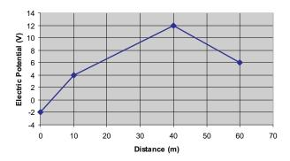
11. [5pt] Suppose the point charge has a mass 3.6 kg and is constrained to move along the x-axis. If the initial speed of the particle is 8.51 m/s along the +x-axis when the particle is located at x = 0, what is the speed of the particle (in m/s) when it is located at x = 60 m?
