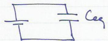
$C_{12} = C_1 + C_2 = 23 \mu\text{F}$
