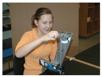
In the final picture, we see the rise of the pendulum as a result of colliding with the steel ball. You will measure the maximum angle reached by the pendulum (here seen to be around 50°). Although the initial collision conserves momentum rather than mechanical energy, the process of the pendulum rising conserves mechanical energy (but not momentum). Using energy conservation, you should be able to determine the speed of the pendulum with the captured ball at the moment just after the collision.
