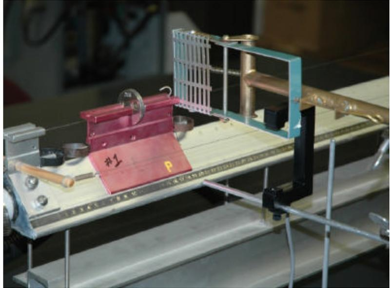
Then, position the trapdoor so that it holds the cart at this position. Finally, adjust the photo-gate shown here so that it will trigger when the trap-door is opened.
