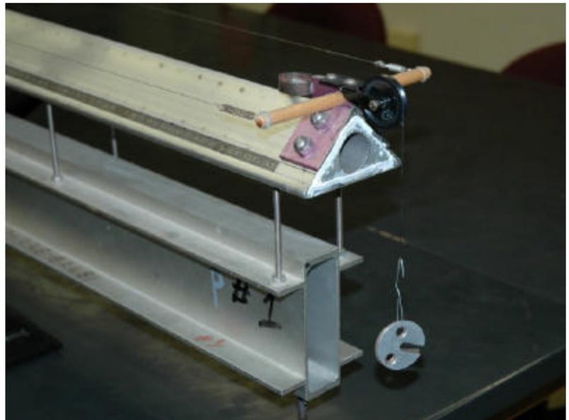
Second, position the cart near the other end of the track. In this image, the front edge of the cart is exactly at the 19 cm mark (it looks like less because this picture was taken at an angle).
