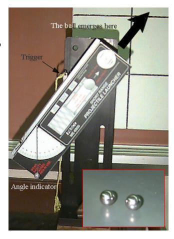
To load the cannon, drop a ball in the tube, and then push it down all the way using the plastic ramrod shown here. Push it all the way in to get the fast setting.
