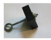
The second method I use for all my Science Olympiad bridges and towers. This method works for both top and bottom loaded bridges. First, I take the leaf out of our old table, and simply lay the bridge over the gap. You can pull two tables close together if you do not have a table with a removable leaf. I then put a loading block on the bridge. The loading block I use comes from Pitsco, and fits the Science Olympiad
